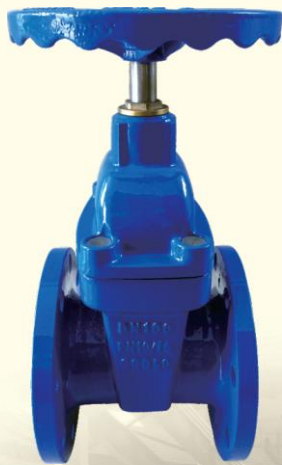
Z45X 软密封暗杆闸阀 NRS Resilient Seated Gate Valve DN40~1000mm
